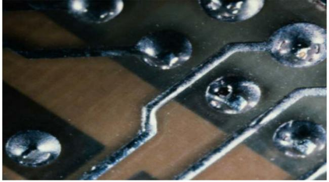
**Dewetting - possible Causes:** Contamination of surface by abrasives Poor plating Poor hot air solder leveling during PCB manufacture
